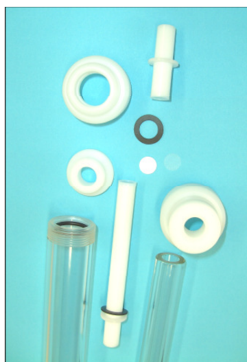
Fig. 1 Parts of the MediaScout® ValiChrom columns.
