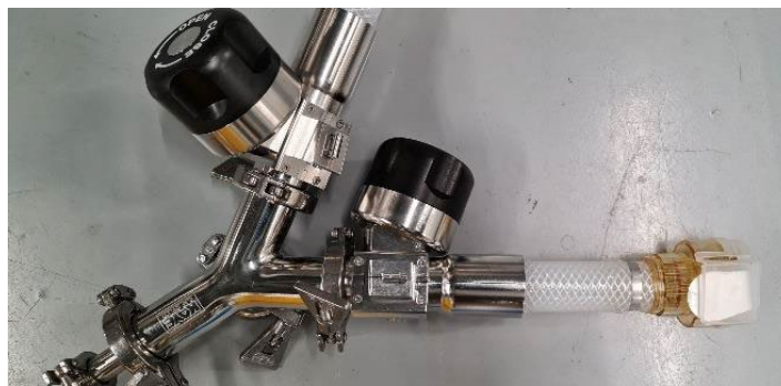
Figure 2. Open valve configuration with dead-ended tubing
