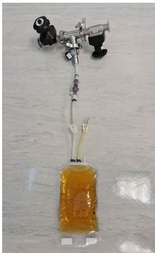
Figure 10. Tested valve shown with adjacent hand valves and TSB in a single-use bag assembly with a Kleenpak connector
