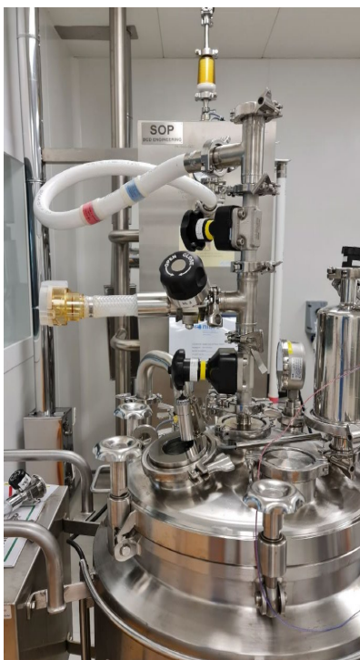
Figure 10. Tested valve shown with adjacent hand valves and TSB in a single-use bag assembly with a Kleenpak connector
