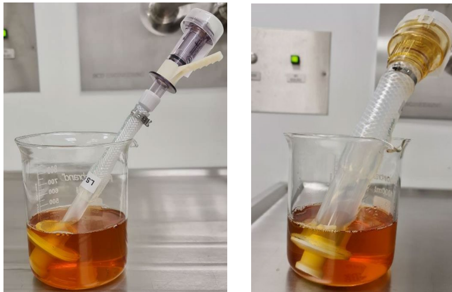
Figure 5. 3/8" ID (left) and 1: ID (right) submerged in B. diminuta suspension
