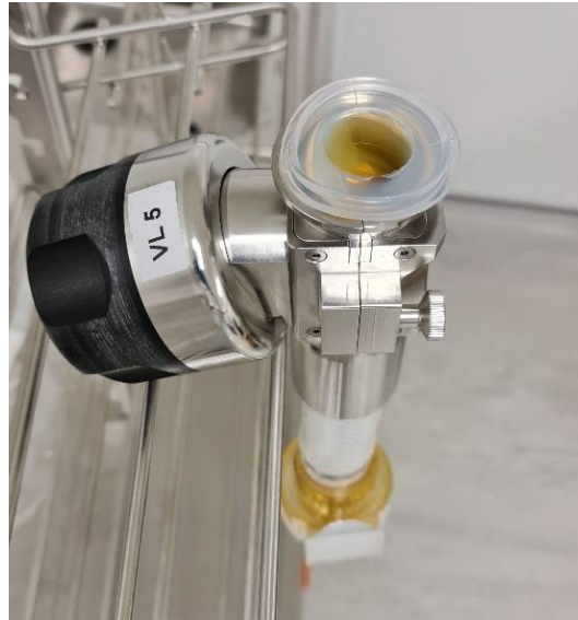
Figure 7. Valve dipped in bacterial suspension for 5 minutes
