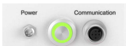
Figure 1: Back of KONDUiT, green power light on the On/Off button indicates if KONDUiT is receiving power.
