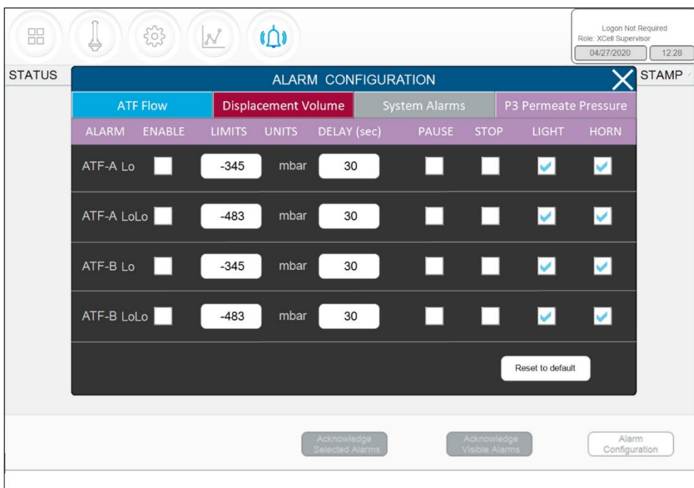
Figure 55. Default values for P3 Permeate Pressure Alarms
