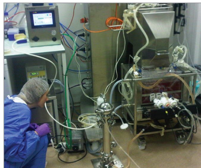
Microcarrier-based perfusion in a single-use ATMI bioreactor
