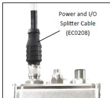
Figure 32. Connect Power and I/O Splitter Cable (EC0208) to FlowVPX Head
