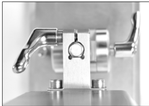
Figure 24. Install FlowVPX Head on mounting post
