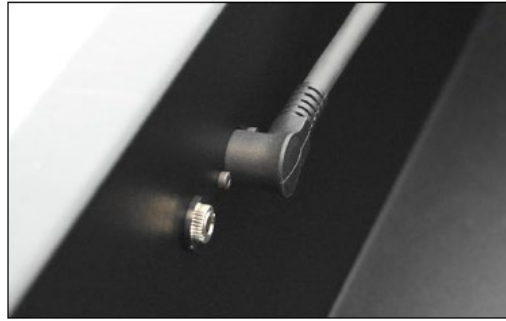
Figure 28. Detector Cable in sample compartment
