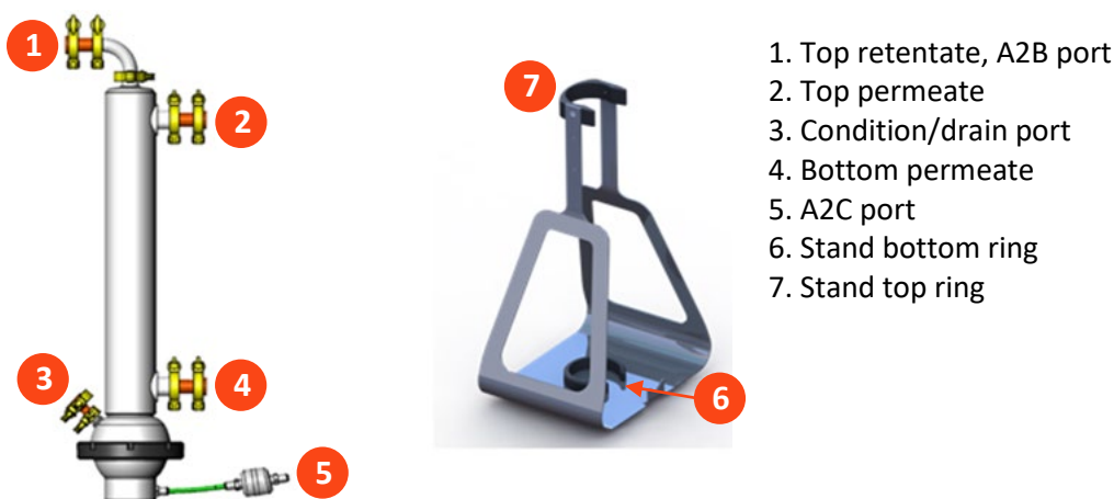
Figure 3. XCell ATF 6 Single-use Device ports and stainless steel stand
