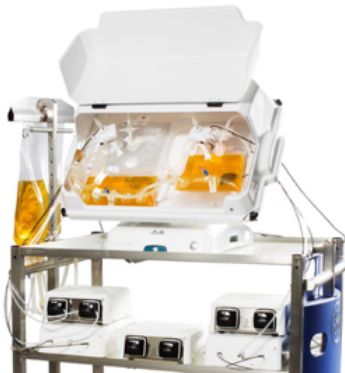
Fig. 1 Single-use intensified perfusion-based bioproduction process development in a Perfusion Cellbag™ bioreactor (GE Healthcare).
