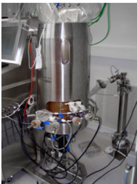
Fig. 2 Hybrid continuous bioproduction accomplished in a GE Healthcare XCellerex™ XDR bioreactor (left) supported by a Repligen XCell™ ATF System (right).
