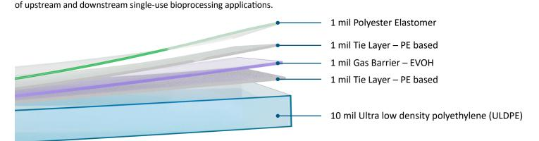
Repligen ProConnex® RG-V Film is a single-ply, 5-layer, 14 mil thick film developed specifically to meet the stringent quality standards
